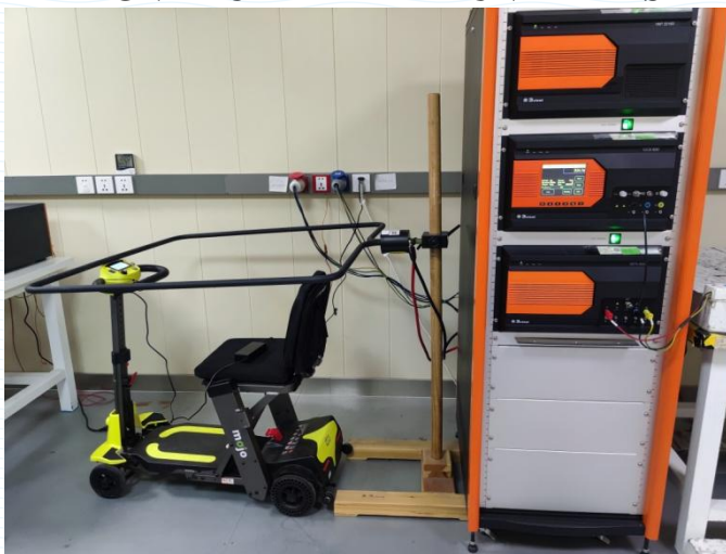
Figure 9 MAGNETIC FIELD IMMUNITY TEST
