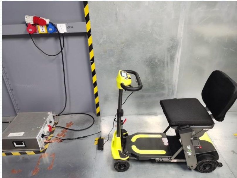
Figure 1 CONDUCTED EMISSION TEST
