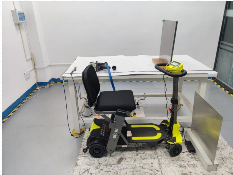
Figure 5 ELECTROSTATIC DISCHARGE TEST
