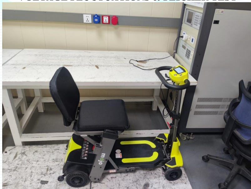
Figure 4 HARMONIC CURRENT EMISSION TEST VOLTAGE FLUCTUATIONS & FLICKER TEST
