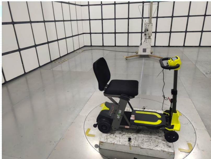
Figure 2 RADIATION EMISSION TEST
