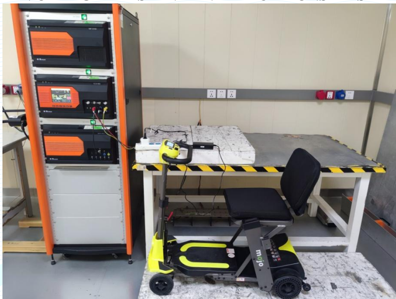
Figure 7 ELECTRICAL FAST TRANSIENT/BURST TEST SURGE TEST VOLTAGE DIPS AND INTERRUPTIONS TEST
