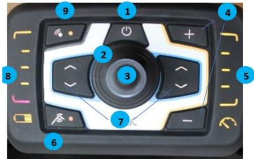
When pressed speed up and down buttons simultaneously the device mode turns from standard wheel mode to large wheel mode. The mode is displayed on the User Panel by the way speed lights are lit. Speed Indicator and drive mode selection display indicates maximum speed level of led bars. Depending on the drive mode selection the speed indicator either shows a solid bar graph or a single point led display.
