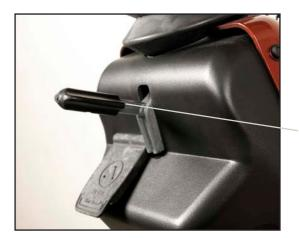
Adjusting the height of the handlebars. Applies to both the 3W and the 4W model.
