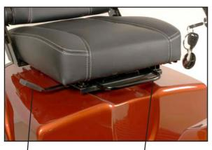
Release lever for seat rotation. Release lever for seat forward/back.
