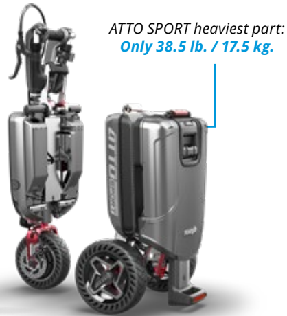
SPLIT MODE Separates into 2 lightweight parts
