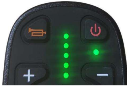
Figure 2 - Power indicator on the companion control unit
