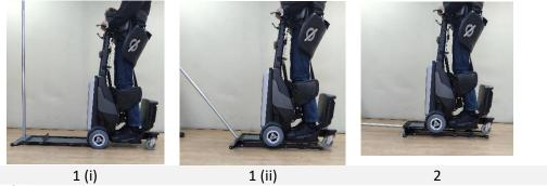
WARNING: The lifting jack has moving parts which can easily pinch an object with severe force. Placing fingers or other body parts near the lifting jack while on the floor or while being carried can lead to serious injury. To avoid pinching, always keep all body parts away from the lifting jack. Do not place any body part in between the small spaces of the jack. Always detach the lever from the lifting jack when not in use.
