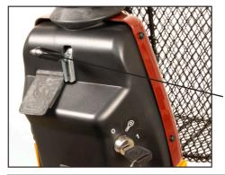
Adjusting the height of the handlebars.
