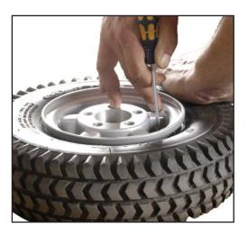
Remove the valve cap and use a screwdriver or similar to open the valve so that the air can be released.
