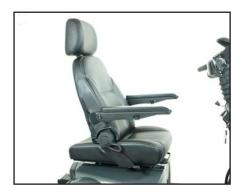
The depth of the seat can now be adjusted by sliding the seatback forward and back.
