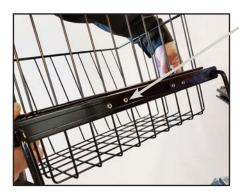
The basket with the mounting bracket. You have to adjust the width by loosening the four screws - pull or push untill the width fits.
