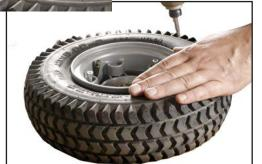
In this way the tube will not get jammed, when the flange is mounted again.
