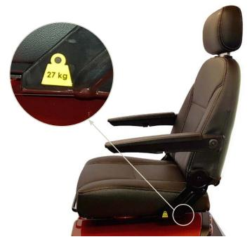
This is our standard Ergo2 45 cm seat, the heaviest part of the X1 to remove. The label showing the seat's weight is located as shown above.
