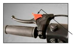
When using the hand brake as a parking brake, lock it in braking position by pressing the button in while applying the
