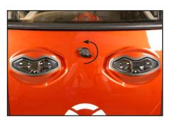
Open the front cover, by turning the handle 90° counter clockwise, and pull.
