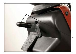
Adjusting the height of the handlebars.
