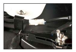
Remove the headlight. Detach the plug, and it is free to change.
