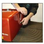
Remove the thumbscrew and remove the battery cover.
