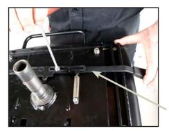
Placement of lever for rotating the seat on the left-hand side
