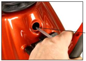
Adjusting the height of the handlebars.
