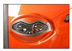
The headlight can be adjusted up/down by turning this screw.
