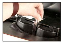
The headlight is attached with a fitting on the back of the screen. A single finger screw holds it firmly in place. Remove the screw.
