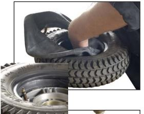
Replace or patch the tube. Ensure that there are no foreign objects in the tyre before the tube is replaced.
