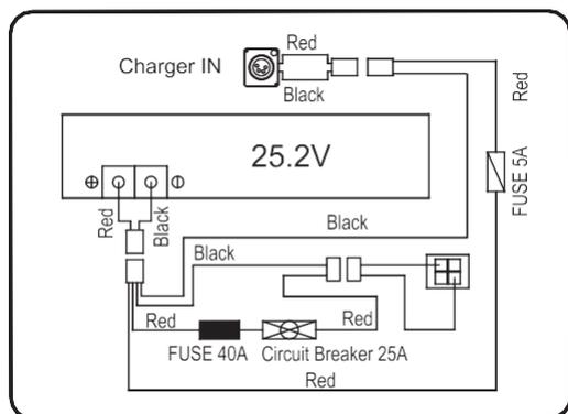
Lead-acid battery - Circuit diagram
