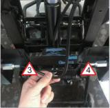
The right folding unit locking pin (shorter steel cable) passes inside the sliding base.
