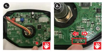
• After a change of battery type, be sure to change the steering head charger socket and the battery pack charger socket. See *SERVICE-01-6 Steering Head Charger Socket* Repair and *SERVICE-06-1 Battery Pack - Charger* Socket Repair. Do not attempt to modify the charger socket or charger cable connector. This can be very dangerous and have severe consequences.
