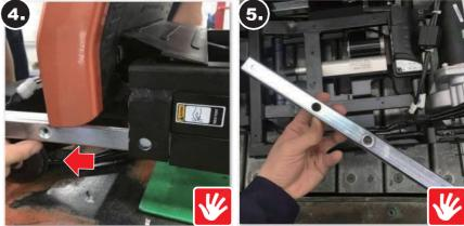
• If the sliding track does not come out easily (Steps 3 and 4), shake the frame or press the folding/ unfolding button several times to fold and unfold. This will push the sliding track out. Be careful to keep your fingers out of the way when doing this to avoid an accident.
