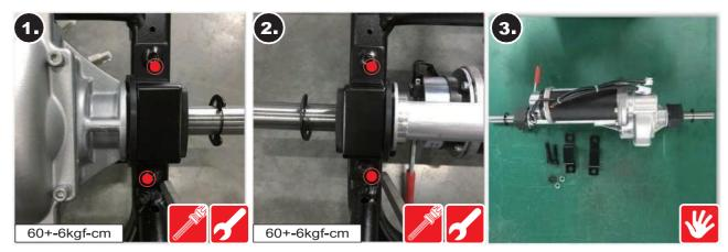
The motor is heavy, and this operation should be given the attention of two people. One can support the motor while the other removes or replaces the bolts, etc. The scooter should be turned over to make this operation easier.
