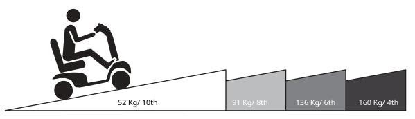
The degree of incline is affected by the weight capacity, speed, grade, and parameters of the scooter.
