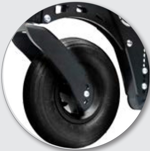
200x50 pneumatic tyre with anti-flutter fork
