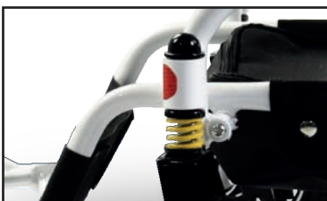
Hi-torque front suspension
